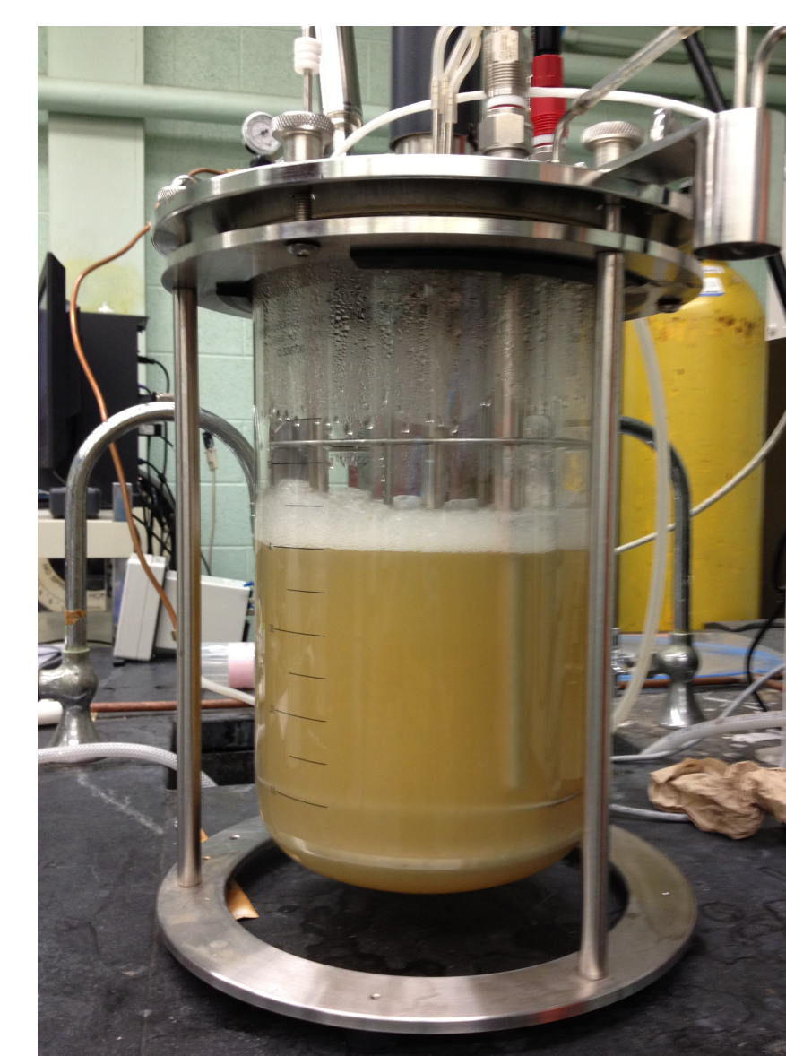
Figure 5. Fermentor culture in 7-liter BIOFLO-110 bioreactor.
